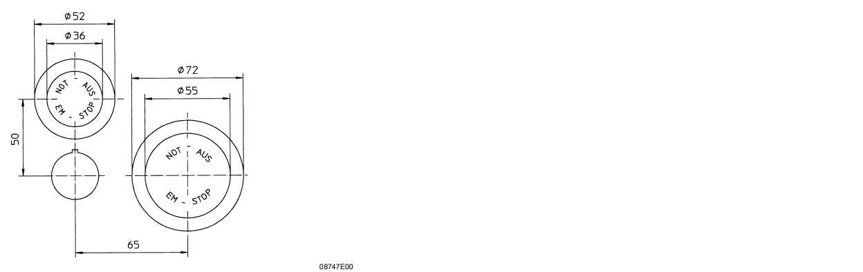
Cut-out for EM-STOP button (8003/...-009, -010, -015)
