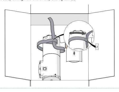
Pull the strap to tilt the unit in vertical position while still in the box.
