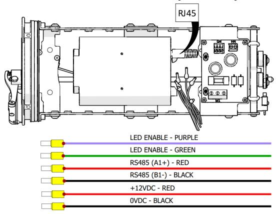
LED ENABLE: connect IR LED activation only on TSP-LED models.
