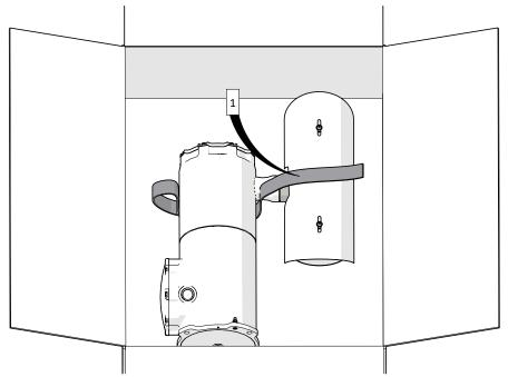
Pass the strap through the end of loop and tighten (2).
