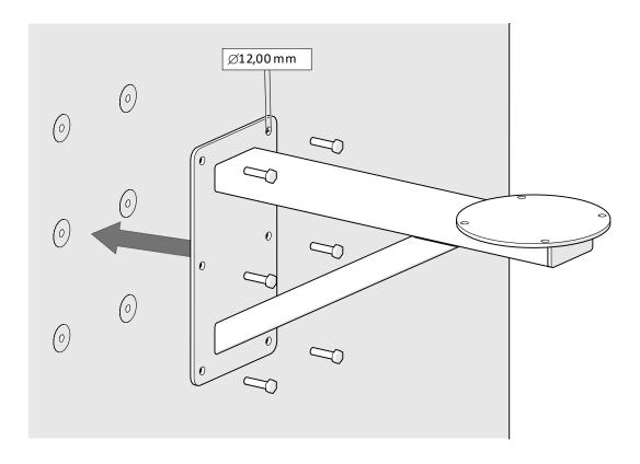
To install the PTZ to the bracket, 4x M10 screws, 4x lock Washer and 4x nuts (provided with the SSBK-L bracket) must be used.
