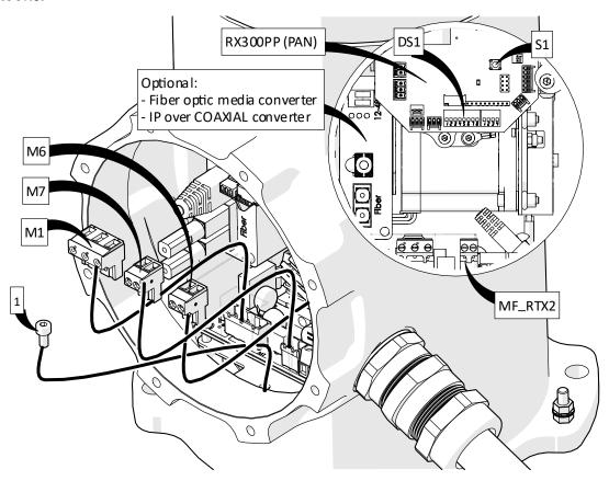
Each plug-in connector is different in shape and/or colour to avoid any wrong connection. The connections should be performed according to the below indications:
