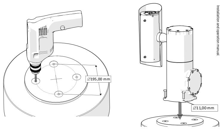
Upon each start-up, the unit will perform a "zero-axis" calibration. "Zero-axis" position is with side flange on the left (cable entry on the back) and camera(s) facing forward. The unit should be installed with the cable gland facing the opposite direction to the zone to be monitored.
