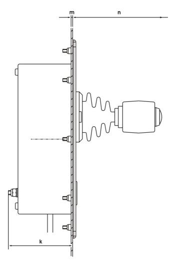
k = depth of cut-out = 60 m = material thickness = up to 6n = design front height = 83
