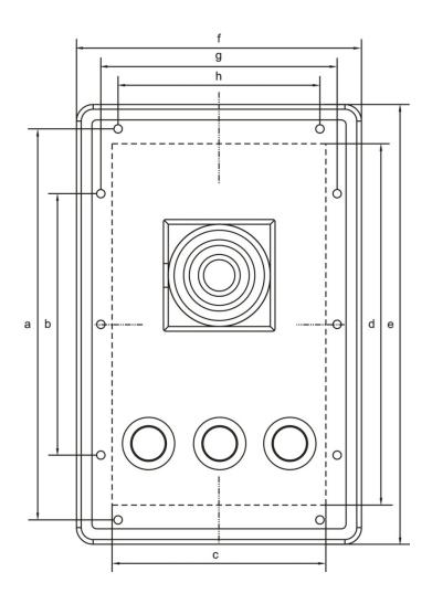
dimensions front plate height (h) = 185е dimensions front plate width (w) = 120 f cut-out width (w) С =  $= 90 (\pm 1)$ cut-out height (h)  $= 152 (\pm 1)$ d distance fitting holes = 164.5а distance fitting holes = 110 b distance fitting holes = 99.5g distance fitting holes = 85
