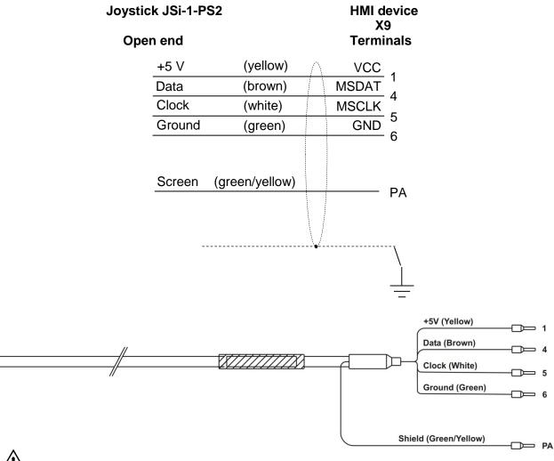
The shielding connection (green/yellow cable) must be connected to the PA terminal block of the HMI devices!
