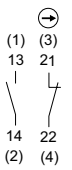
Schematic 8003/143 Positive opening NC/NO The numbers in brackets correspond to the core marking
