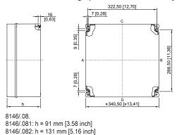
8146/.083: h = 150 mm [5.91 inch] 8146/.084: h = 171 mm [6.73 inch] 8146/.085: h = 190 mm [7.48 inch] 8146/.086: h = 230 mm [9.06 inch]
