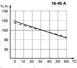
Correction factors for ambient temperatures which deviate from 30  $^\circ\text{C}$
