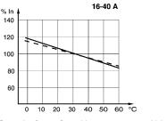
Correction factors for ambient temperatures which deviate from 30  $^\circ\text{C}$
