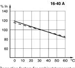
Correction factors for ambient temperatures which deviate from 30  $^\circ\mathrm{C}$
