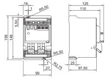
8562/54-...., 2-pole with auxiliary contact and reset function
