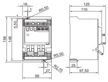
$8562/54\text{--}...,\,2\text{-pole}$  with auxiliary contact and reset function
