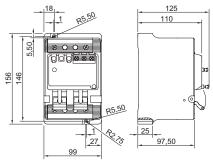
$8562/54\text{--}....,\,2\text{-pole}$  with auxiliary contact and reset function
