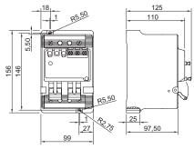
$8562/54\text{-}....,\,2\text{-pole}$  with auxiliary contact and reset function
