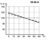
Correction factors for ambient temperatures which deviate from 30  $^\circ\mathrm{C}$
