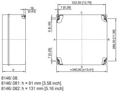
8146/.082: h = 131 mm [5.16 inch] 8146/.083: h = 150 mm [5.91 inch] 8146/.084: h = 171 mm [6.73 inch] 8146/.085: h = 190 mm [7.48 inch] 8146/.086: h = 230 mm [9.06 inch]
