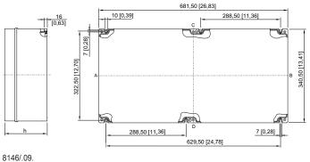
8146/.09. 8146/.091: h = 91 mm [3.58 inch] 8146/.092: h = 131 mm [5.16 inch] 8146/.093: h = 150 mm [5.91 inch] 8146/.095: h = 190 mm [7.48 inch]
